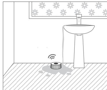
Put the sensor in the area where water leakage may happen.
